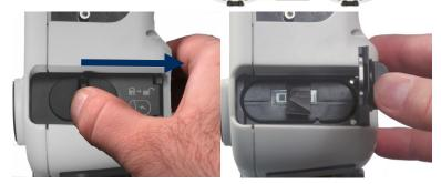
Allow the Xpress to charge initially for at least 5 hours to reach a full charge. Other than charging the batteries, no user maintenance of the batteries is required.
