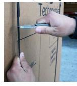
Use a #2 Phillips screwdriver to remove the four drywall screws and washers (two on each side).
