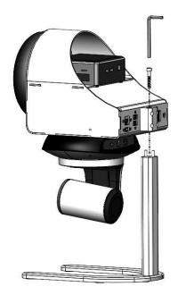
**Step 2:** Align the TVPro One assembly to the completed stand, insert the M6 Socket Head Screw, and tighten with the M5 hex key.
