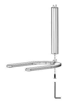
**Step 1:** Align Vertical Mounting Post to the U-Base using the protruding locating pins and insert the M6 Flat Head Screw and tighten with the included hex key.
