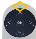
Top LED is solid green when paired and connected.
