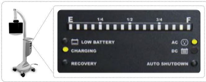
The battery charge indicator is located on the Lite 5 on the side of the storage compartment.
